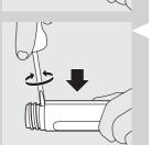
**3** Remove the screwdriver and repeat the above instruction using the other slot located on the opposite side of the handle. Twist the blade and the housing will continue to split.
